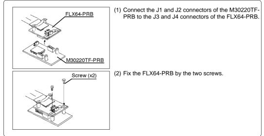
Figure 3.3 Connecting pod probe M30220TF-PRB
